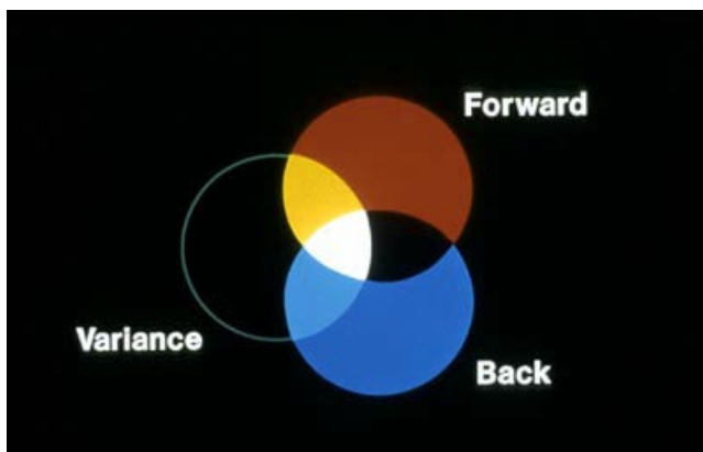
Figure 4.18 When variance is detected, hues of green may be added to the red and blue flows, resulting in shades of yellow, white, and blue-green (cyan).
